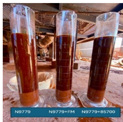
Figure 5. Plant jar tests.
